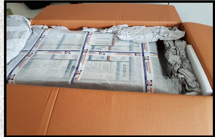
Server packed with Foam Sheet, Air bubble and empty places are Stuffed with Tissue paper
